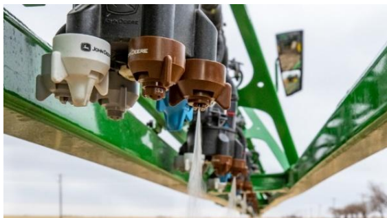
Slika 5.19. ExactApply mlaznice (Izvor: https://www.deere.com/en/technology-products/precision-ag-technology/precision-upgrades/sprayer-upgrades/exactapply-precision-upgrades/ )
