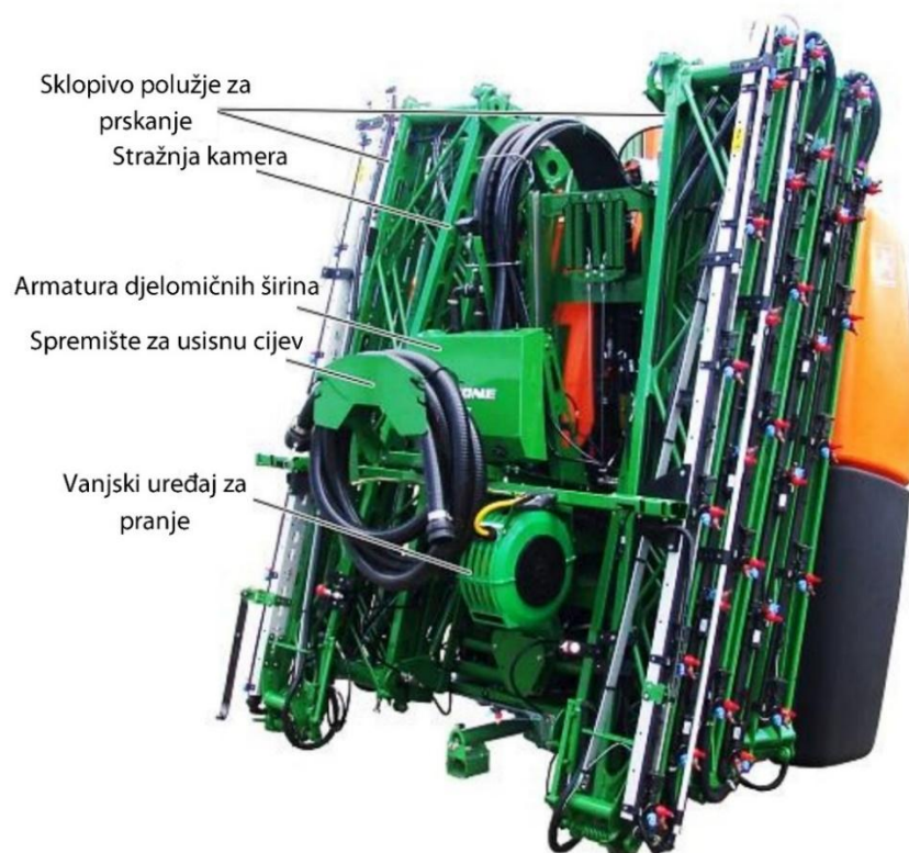
Slika 3.87. Prikaz ugrađenih sklopova prskalice „AMAZONE” UF 2002 (Izvor: https://e-farm.com/en/used-farm-machinery/sprayers/amazone/uf-2002-15/du8cqzw/ )
