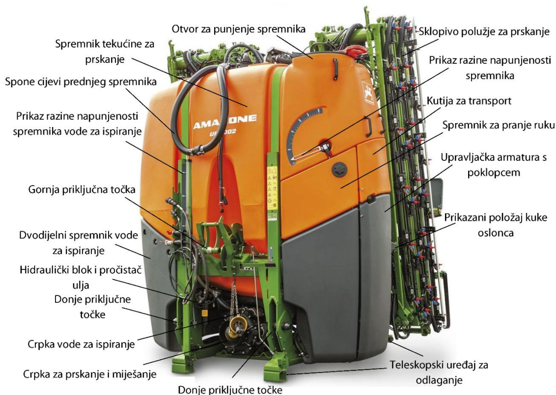
Slika 3.87. Prikaz ugrađenih sklopova prskalice „AMAZONE” UF 2002 (Izvor: https://e-farm.com/en/used-farm-machinery/sprayers/amazone/uf-2002-15/du8cqzw/ )
