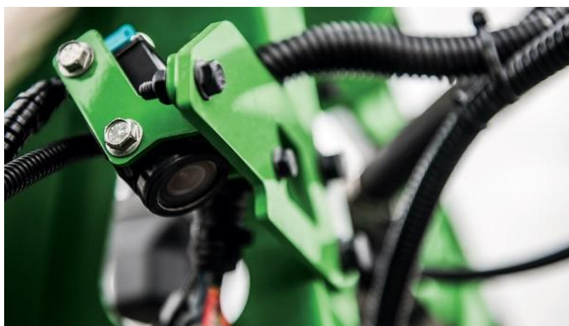
Slika 5.21. Integrirana kamera za snimanje stanja (Izvor: https://www.deere.com/en/sprayers/see-spray-select/ )
