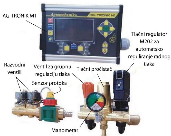
Slika 4.64. Regulator tlaka PR9 (Izvor: https://agricom.pt/en/383-control-units )
