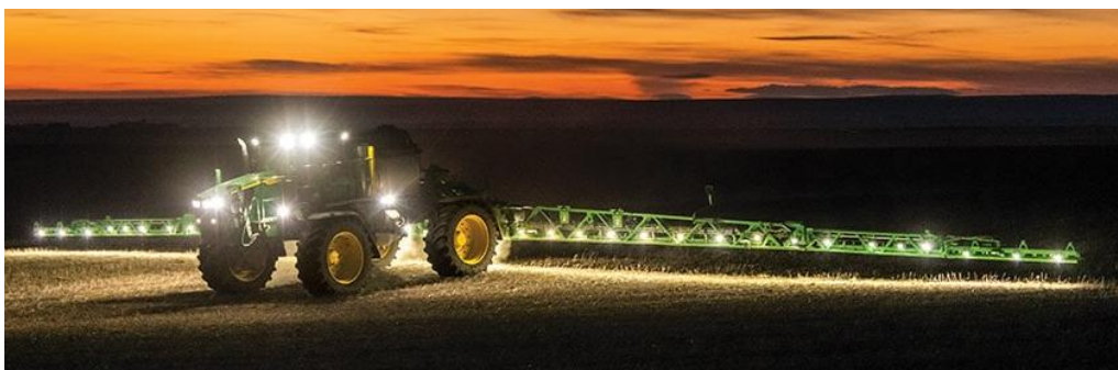
Slika 5.23. See&Spray Select sustav u noćnom radu (Izvor: https://www.deere.com/en/sprayers/see-spray-select/ )
